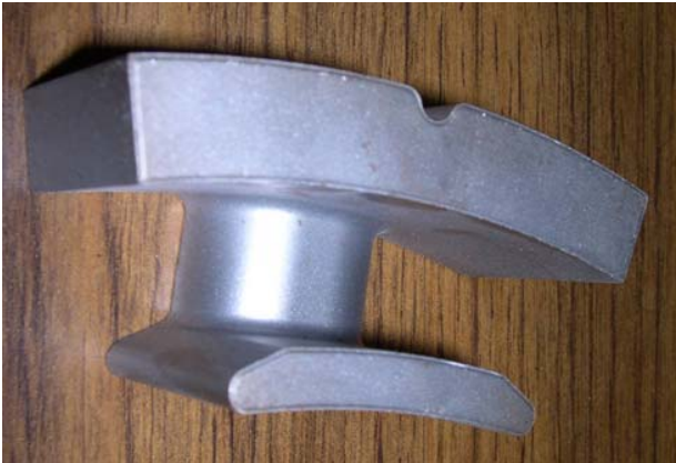
Figure 1: Single tooth with extended back iron and tip.
